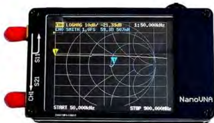
NanoVNA vector network analyzer
