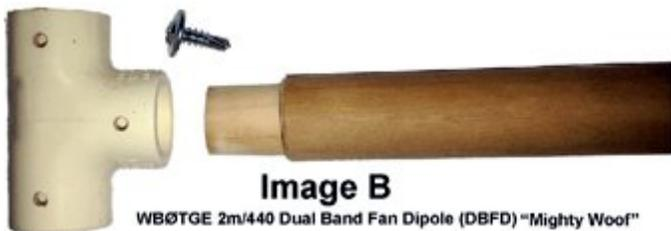
Looking at Image B, drill three 1/8" pilot holes on one side of the plastic tee about 1/4" from the ends of the openings. The image shows the 1/2" self-tapping screw used and the hardwood dowel used as the the mounting mast for the antenna. Sand the dowel end to match the inside diameter of the tee. Make it a press fit and long enough to seat completely into the tee opening. The copper pipes and wood dowel are secured to the tee using the self-tapping screws.
