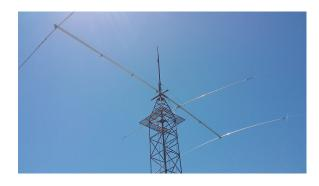
This is a homebrew, shortened 3 element, 40 meter mono bander. The antenna is made from 3 different antennas.
